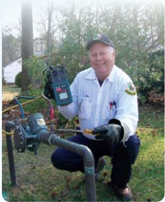
Backflow Technician testing backflow device on irrigation system
