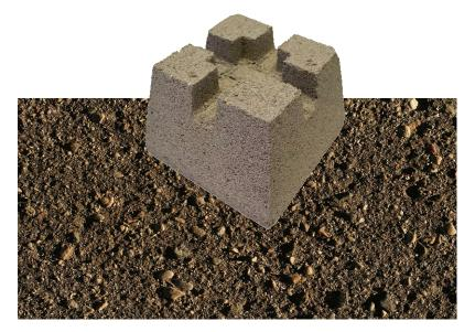
• If less than 200 square feet, and less than 20" above grade (measured from any point within 36"), deck joists are permitted to bear directly on precast concrete pier blocks at grade. Beams and posts are NOT permitted to be supported this way.
