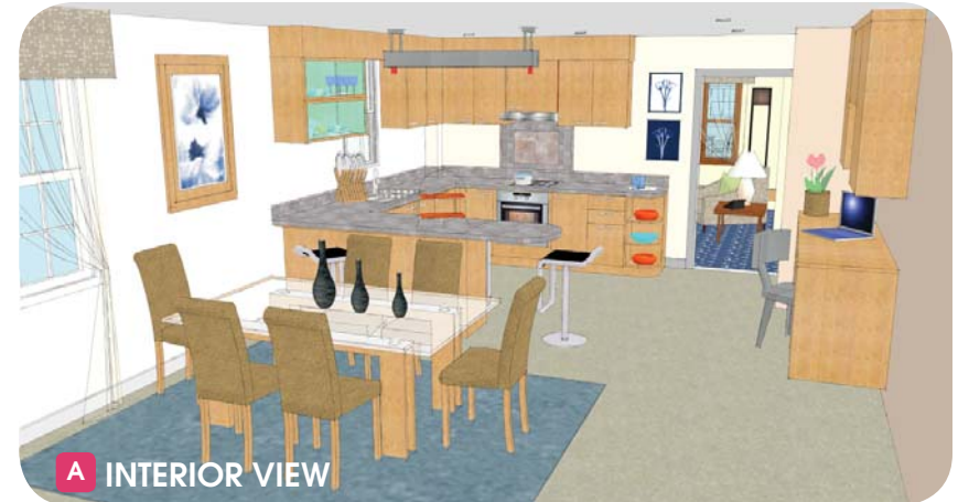
A INTERIOR VIEW By looking towards the front of the house from the corner of the new family room, the open floor plan of the newly enlarged kitchen and dining area shows how a new gathering and entertaining space can be created. The kitchen is expanded into the former dining space and part of the new addition provides a new dining area. The former laundry space is enlarged to create a mudroom/laundry with a door to the new deck.
