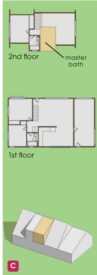
shed-roofed dormer doubled in size
