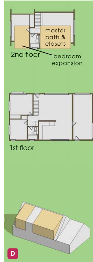
single shed-roofed dormer expanded to full-width
