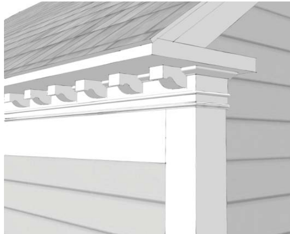
Adding molding to the cornice provides more visual interest and is appropriate in Cape Cod and Colonial Revival style neighborhoods.
