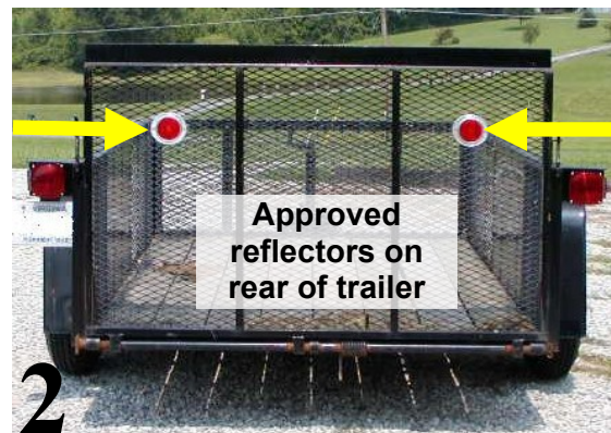
PHOTO 2: NO VIOLATION - This trailer has two reflectors on the rear.
