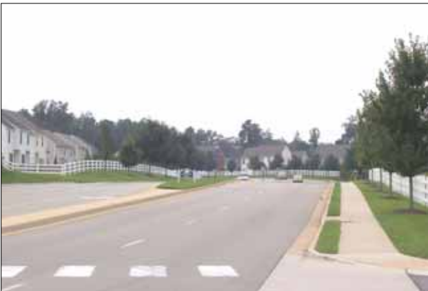
A fence and sidewalk provide Territoriality and Access Control into a neighborhood in Henrico County, VA.
