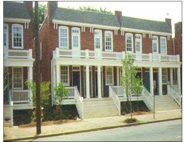
This design in Richmond, VA encourages interaction of neighbors due to the front porches. Natural Surveillance opportunities have been created, and the change in elevation between the porch and sidewalk defines public and private space change.
