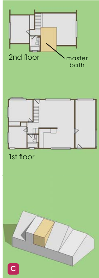
shed-roofed dormer doubled in size
