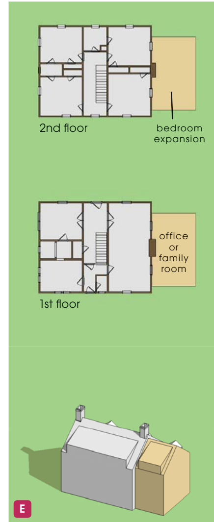
two-story, side addition with gable roof and rear shed dormer
