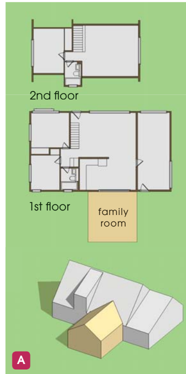
one-story, gable-roofed rear addition
