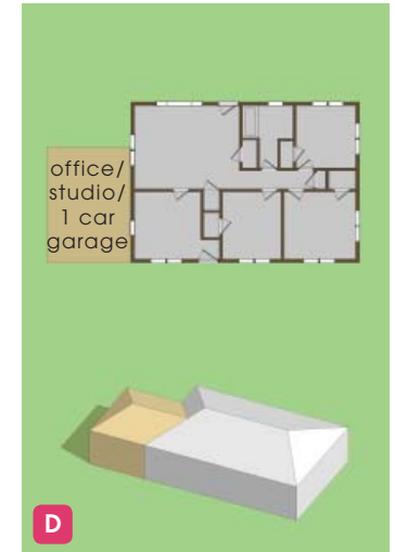
D one-story, hipped roof side addition
