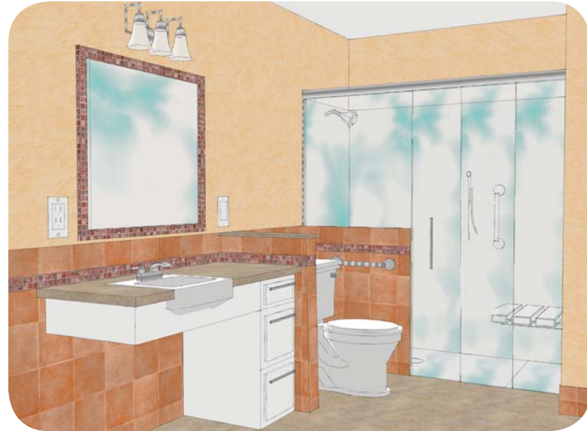
This bathroom view shows how an accessible sink, grab bars, and a shower with a wide door and a fold-down seat can be easily incorporated into a universal design.
