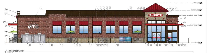
TYPICAL EXTERIOR ELEVATION NOTES: ALL LIGHTS SHOWN ABOVE AND/OR BELOW DOORS OR WINDOWS ARE TO BE CENTERED ON THE DOOR OR WINDOW UNLESS NOTED OTHERWISE.
