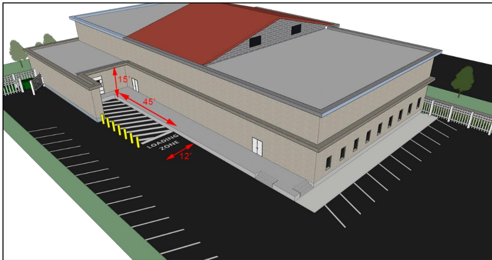
Figure 5124: Loading Area Configuration
