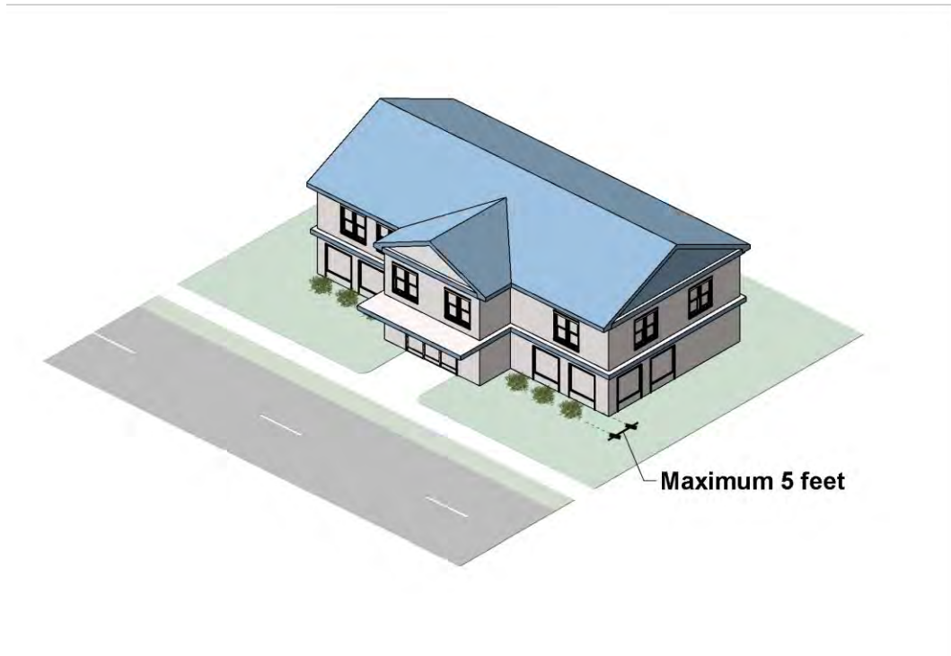
Figure 5309A: Foundation Planting Requirements
