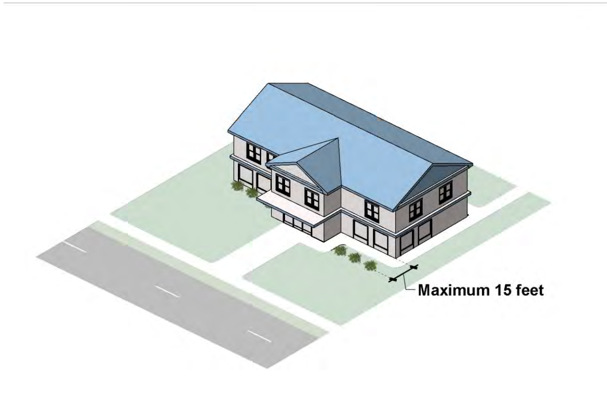
Figure 5309B: Foundation Planting Requirements with Sidewalk
