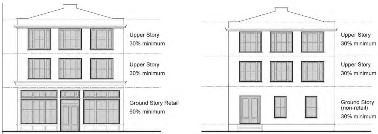
Figure 3840B: Illustration of Façade Transparency Requirements
