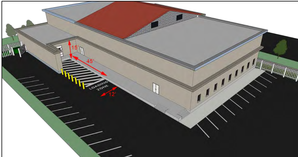
Figure 5124: Loading Area Configuration
