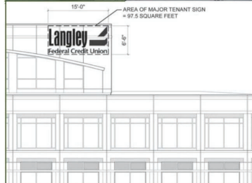
An example of major tenant signage on a mid-rise building. Maximum size of major tenant sign is 150 square feet.
