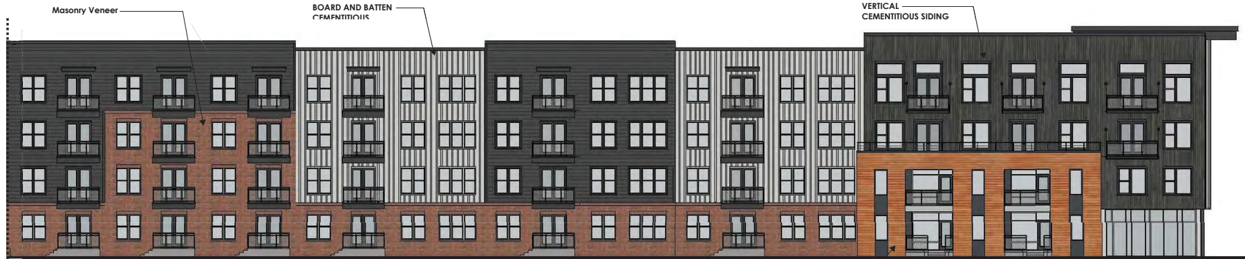
2 Building 1- Partial North-West Elevation Scale: 1" = 20'
